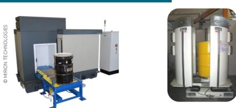
Passive neutron system for radioactive drums
