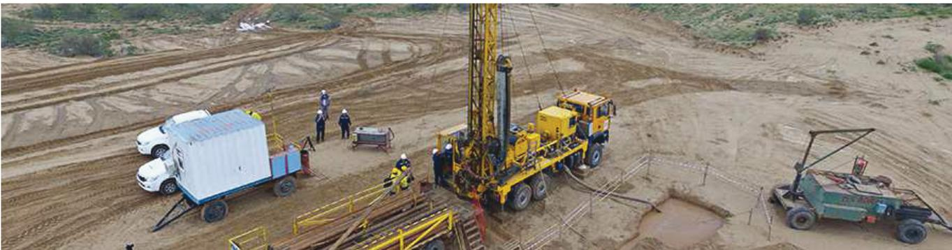
Development of the two mining sites, located approximately 60 kilometers apart, started in April 2004 after the signature of agreements between the two shareholders. The in situ recovery (ISR) technology was chosen to solubilize the uranium directly in the rock.
